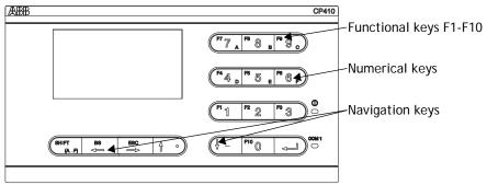
The Functional or Auxiliary Keys F1- F10 can be defined in CP400Soft. They can, for example, be used to set a controller bit or register, to change a screen or to display a password table. Please see the CP400Soft User's Manual for details.
