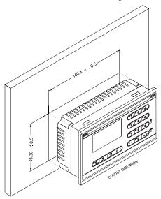
2. Mount the operator terminal into the cut-out. Insert the fixtures to the holes on the unit and fasten the screws into the front panel. Do not tighten the screws with too much force or it may cause the deformation of the operator terminal.
